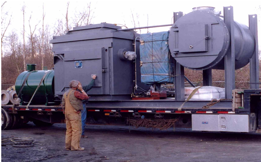
Small BOS systems can be skid mounted
